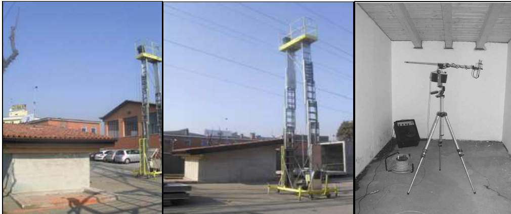
Figure 9: full-scale cell set up: source's position (left, centre); reverberation time measurements (right)
