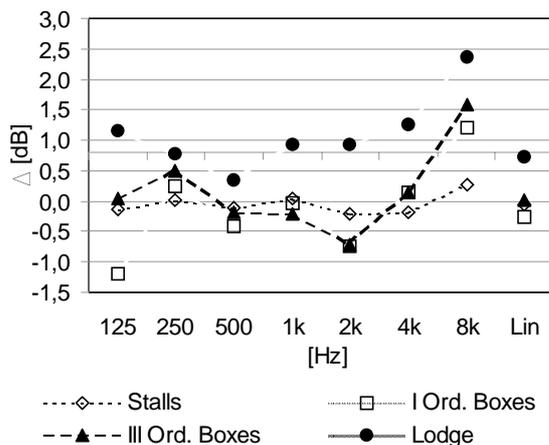
**FIGURE 4.** Difference between  $L_{eq}$  measured in 2001 and in 1997. Data are normalized with respect to the average value of the five points in the stalls which were closer to the source.
