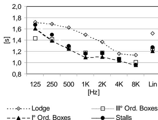
**FIGURE 1.** Plot of reverberation time RT20 measured in 2001. Data averaged according to respective groups of receivers.
