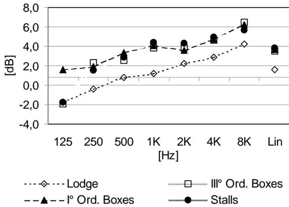
**FIGURE 2.** Plot of clarity C80 measured in 2001. Data averaged according to respective groups of receivers.
