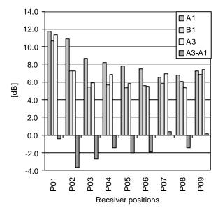
Fig. 6 – Measured data for the parameter G in the stalls.
