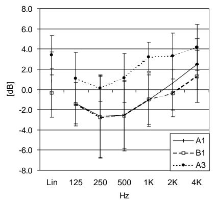
Fig. 5 – The course of the clarity C80 in the stalls for the different postions of sound source. The error bars refer to one standard deviation.
