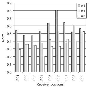
Fig. 7 – The values of lateral fraction LF in the stalls.
